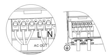
**Note:** The grounding wire shall be as thick as possible (cross-sectional area is not less than 4mm<sup>2</sup>). The grounding point shall be as close as possible to the solar charge inverter. The shorter the grounding wire, the better.
