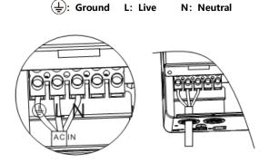
③ Properly connect the AC output wire according to the wire sequence and terminal position shown in the figure below. Please connect the ground wire first, and then the live wire and the neutral wire. The ground wire is connected to the grounding screw hole on the cabinet through the O-type terminal.
